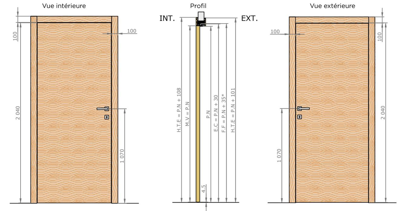
H.T.I = Hors Tout Intérieur | M.V = Mesure Vantail | P.U = Passage Utile
