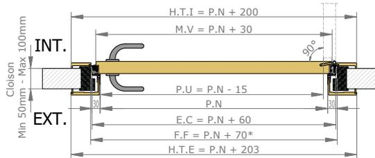
H.T.I = Hors Tout Intérieur | M.V = Mesure Vantail | P.U = Passage Utile
